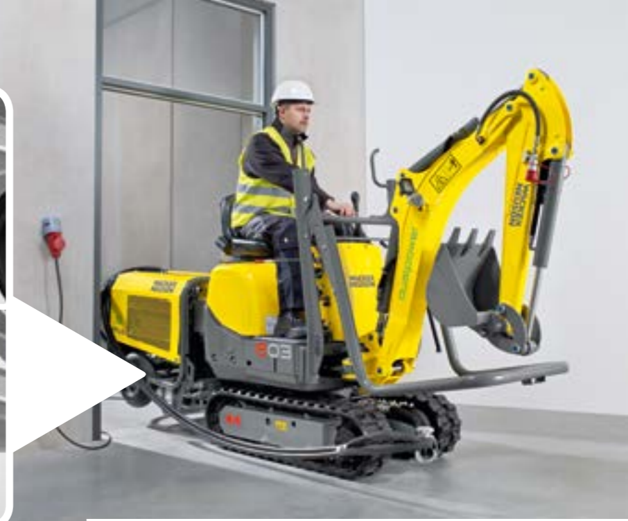
Easy to transport: Two openings are inset in the dozer blade in which the HPU8 can be suspended for transport. The dimensions of the 803 and the HPU8 are perfectly matched to each other so that the team can easily drive through narrow doorways.
